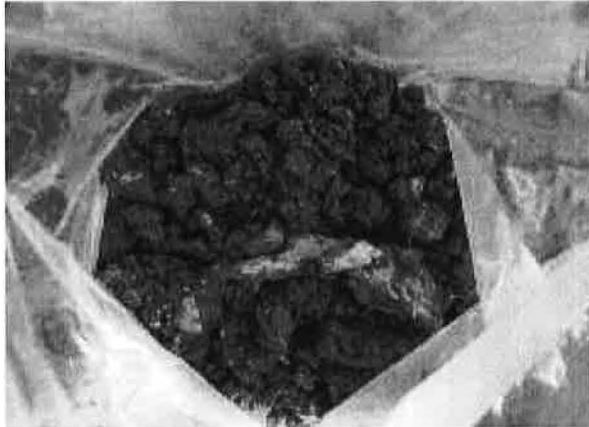
D-1 Borehole B5 cuttings 0.50-0.60 mbgl
