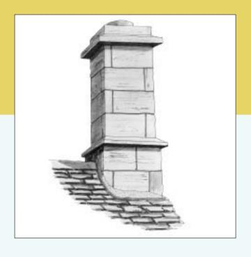
Together with dormer windows, chimneys are one of the most important features of traditional Cotswold buildings. These typical examples of local craftsmanship enliven roofscapes and still provide a practical means of disposing of flue gases. This is a guide to their conservation, and to the design and detailing of new chimneys in the traditional style.
