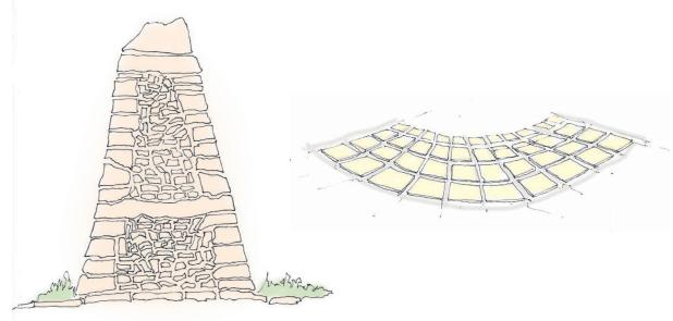
Figure 43: Example showing the construction of dry-stone wall.
