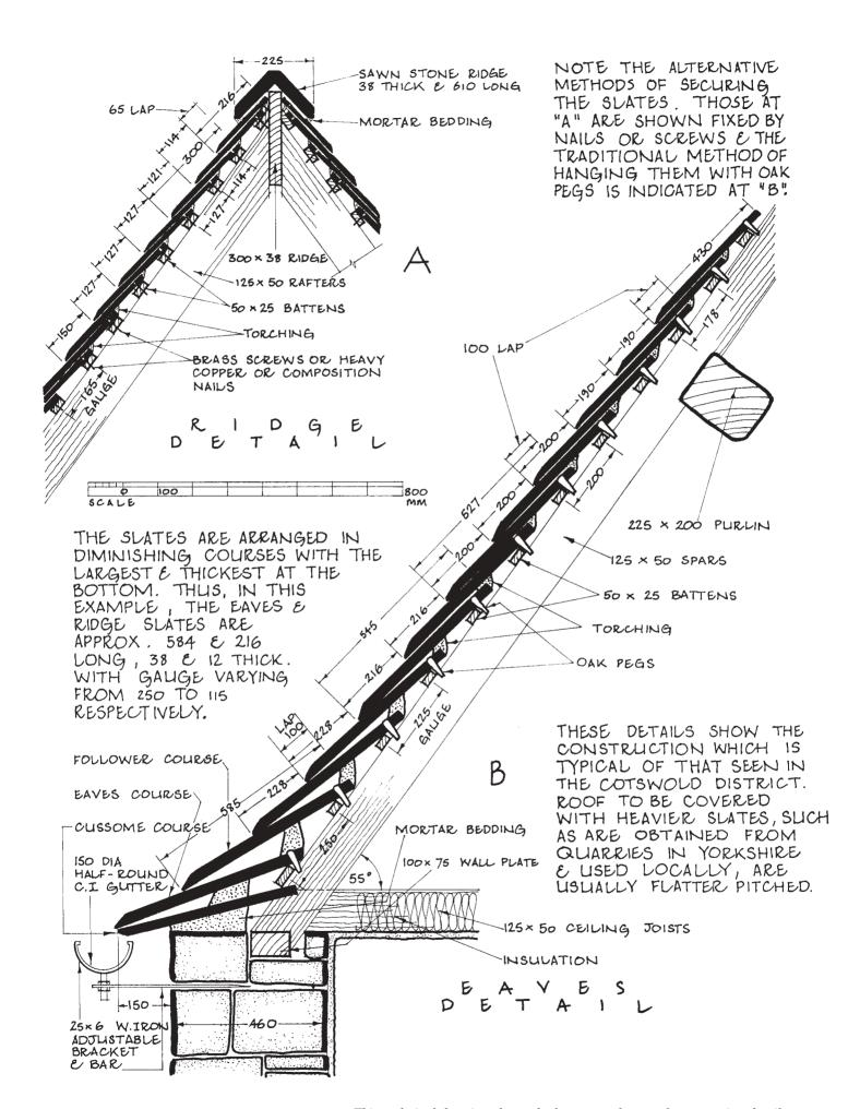
This technical drawing shows the key stone slate roof construction details, especially the eaves and ridge, and the use of diminishing courses.
