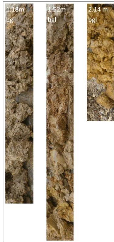
Figure 7. Continuous auger cores through the base of trench-BH3. From left to right: a homogenised ‘trample’ unit; a heterogeneous oxidised clay unit; sandy and clayey terrace gravels.
