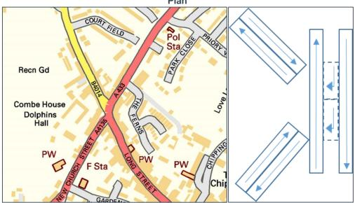
The junction has two minor arms in close proximity (both junctions are on the western side of the A433). There are two right hand turn lanes (one for each junction) for vehicles turning from the A433 London Road to New Church Street and from the A433 London Road to the B4014.
