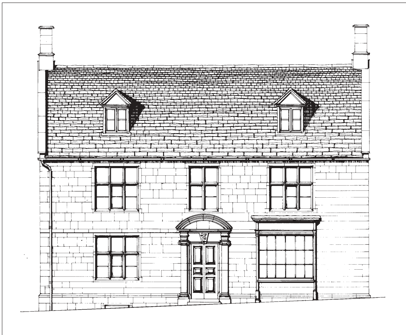
A scale drawing of the front elevation of Halfway House, a fine early-Georgian town house in the High Street dated 1732. The shop window was added in the Regency period.
